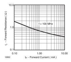
Figure 1. Forward Resistance vs. Forward Current
