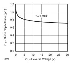
Figure 2. Diode Capacitance vs. Reverse Voltage
